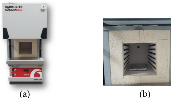
Figure 2: (a) CarboliteGero CWF 1200 Heating Chamber, (b) Sample fibres are inside the brass plate in the furnace.
