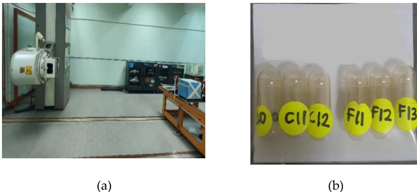
Figure 3: Irradiation setup for basic dosimetric characterisation of fabricated Ge-doped optical fibres (a) a gamma Cobalt-60 machine, (b) Samples fibres CF and FF in gelatine capsules.
