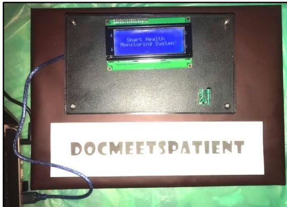
Figure 12: Shows the prototype Smart Health Monitoring System (DocMeetsPatient)
