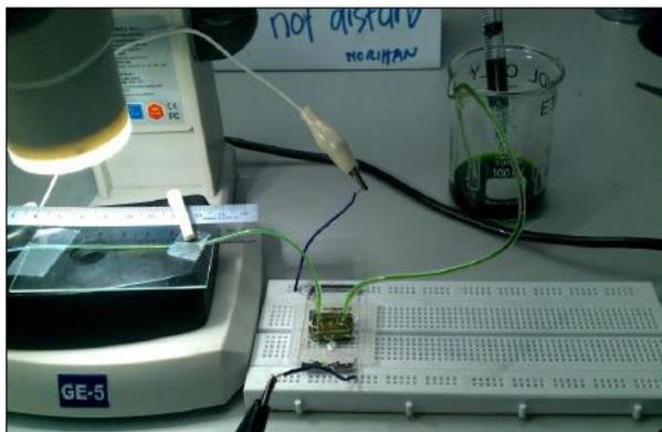
Figure 9: Actual functionality test of thermo pneumatic micropump
