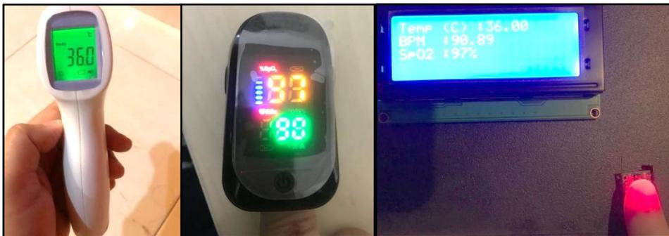
Figure 17: Shows a comparison of body temperature, pulse rate, and blood oxygen levels that have been measured using a real device with readings measured using a designed Smart Health Monitoring System.
