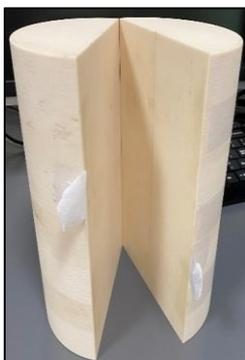
Figure 1: Customized blood equivalent phantom
